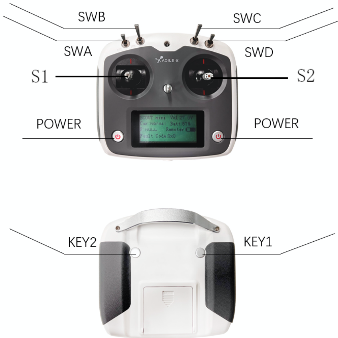
Figure 2.8 Schematic Diagram of Buttons on FS RC transmitter
