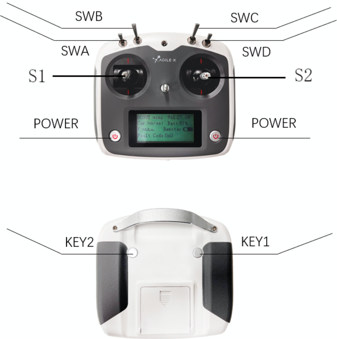
Figure 2.8 Schematic diagram of the FS remote control buttons
