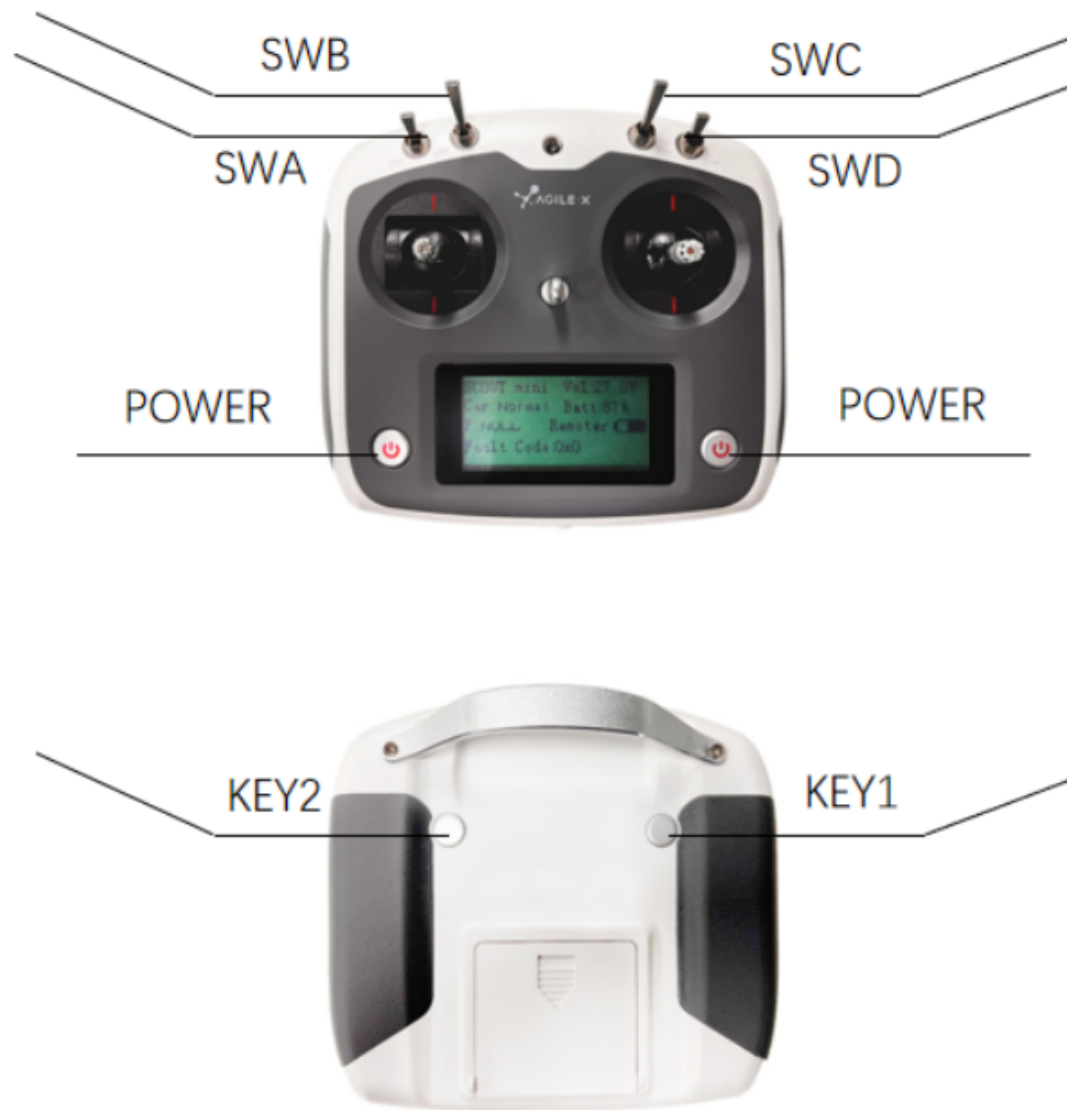
Figure 2.4 Remote controller schematic
